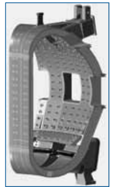
Fig.2 One of the 9 sectors (40 degrees) of the ITER vacuum vessel. verhoeven@rijnhuizen.nl
