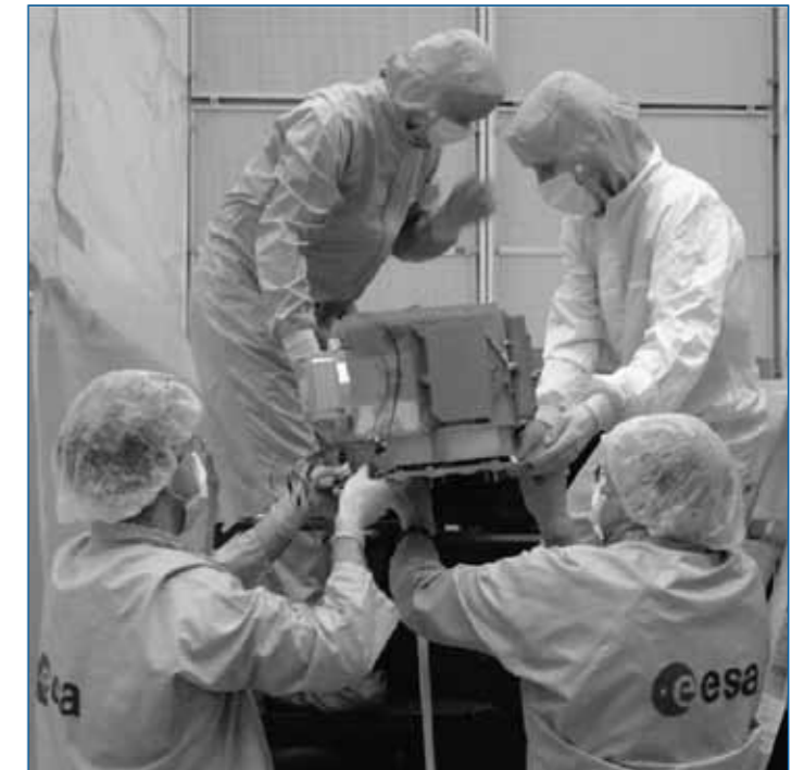
Figure 1. Vibration test preparations on the JWST MIRI flight model, the Mid Infrared Spectrometer Main Optics Box for the James Webb Space Telescope, currently scheduled to be launched in 2013.
