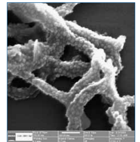
FIG. 1. Carbon nanotubes studded with cobalt-iron nanoparticles. Sample courtesy of Dr. Andreas Huetten, University of Bielefeld, Germany.
