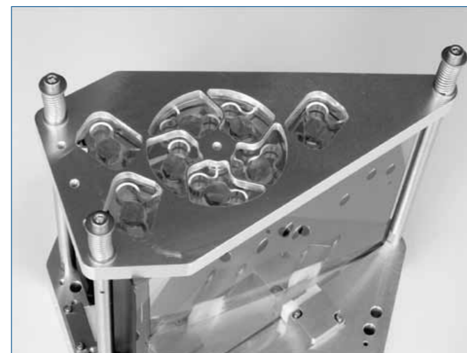
Figure 2. X-shooter prism mount for use in a vacuum cryogenic environment (ESO VLT). Despite the difference in thermal expansion of the mount and the optical material, the prism must remain in position within a few micrometer at any temperature and in any gravity orientation.
