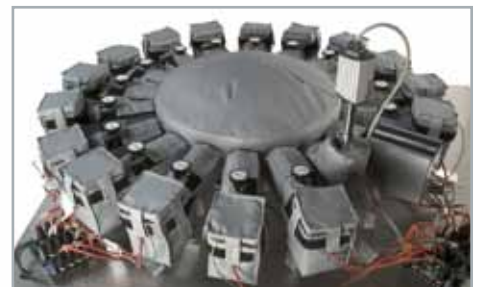
Image detail: UHV vacuum chamber with 16 components in heating jackets connected
