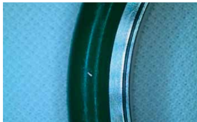
Figure 8 Example of a greased and contaminated O-ring. A particle originating from the stainless-steel clamp commonly used in vacuum interfaces.
