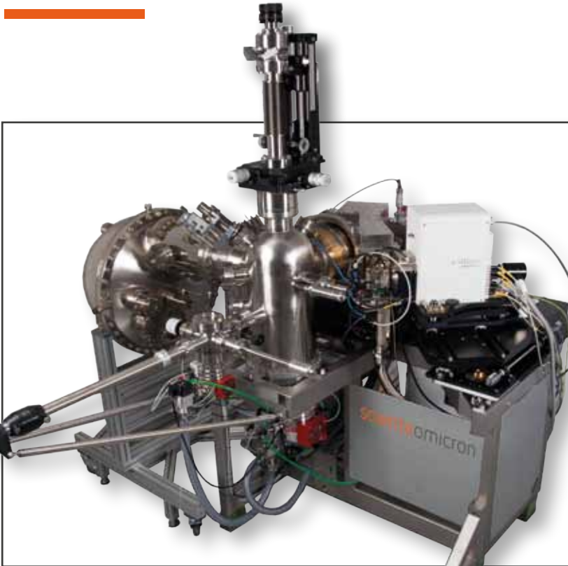
Figure 1. HAXPES using the Ga source offers 5x greater information depth, providing bulk sensitivity that is unavailable using conventional XPS.
