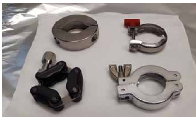
Figure 7 Clamps produce particles during fastening or unfastening. 1. Al double bolts clamp, 2. Cheap stainless steel/brass bolt clamp, 3. Evac chain clamp, 4. Al wingnut clamp).
