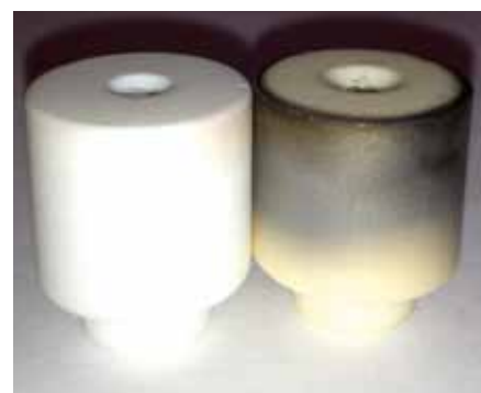
Figure 2 New (left) and more than 50,000 hours of operation (right) insulators are shown with high sputter deposits. SIP pump life time is of the order of 50,000 hours at 10^{-6} mbar.
